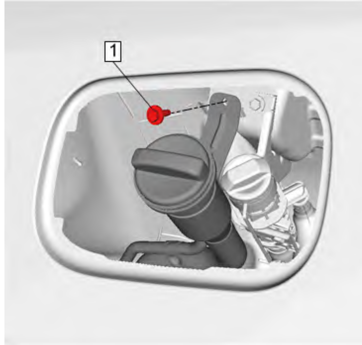
Fig. 101: Fuel Tank Filler Pipe Ground Bolt Courtesy of GENERAL MOTORS COMPANY
