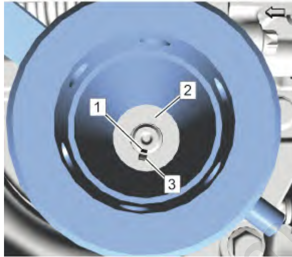
Fig. 216: Fuel Injection Pump Sprocket, Paint Mark And Sprocket Groove Courtesy of GENERAL MOTORS COMPANY
