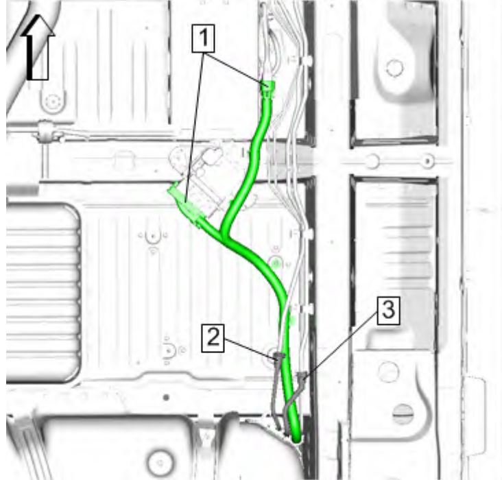
Fig. 78: Fuel Tank Fuel Pump Module Wiring Harness, Fuel Pump Fuel Return Hose And Fuel Pump Fuel Feed Hose
