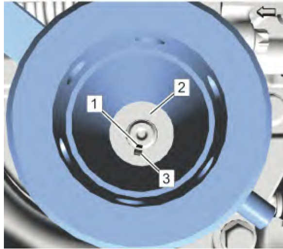
Fig. 249: Fuel Injection Pump Sprocket, Paint Mark And Sprocket Groove Courtesy of GENERAL MOTORS COMPANY
